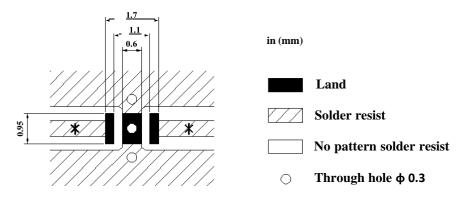
\*Line width to be designed to match 50 $\Omega$  characteristic impedance depending on PCB material and thickness.
