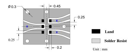
\* Line width should be designed to match  $50\Omega$  characteristic impedance, depending on PCB material and thickness.
