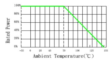
Power rating or current rating is in the case based on continuous full-load at ambient temperature of  $70^{\circ}$ C. For operation at ambient temperature in excess of  $70^{\circ}$ C, the load should be derated in accordance with figure of derating Curve.
